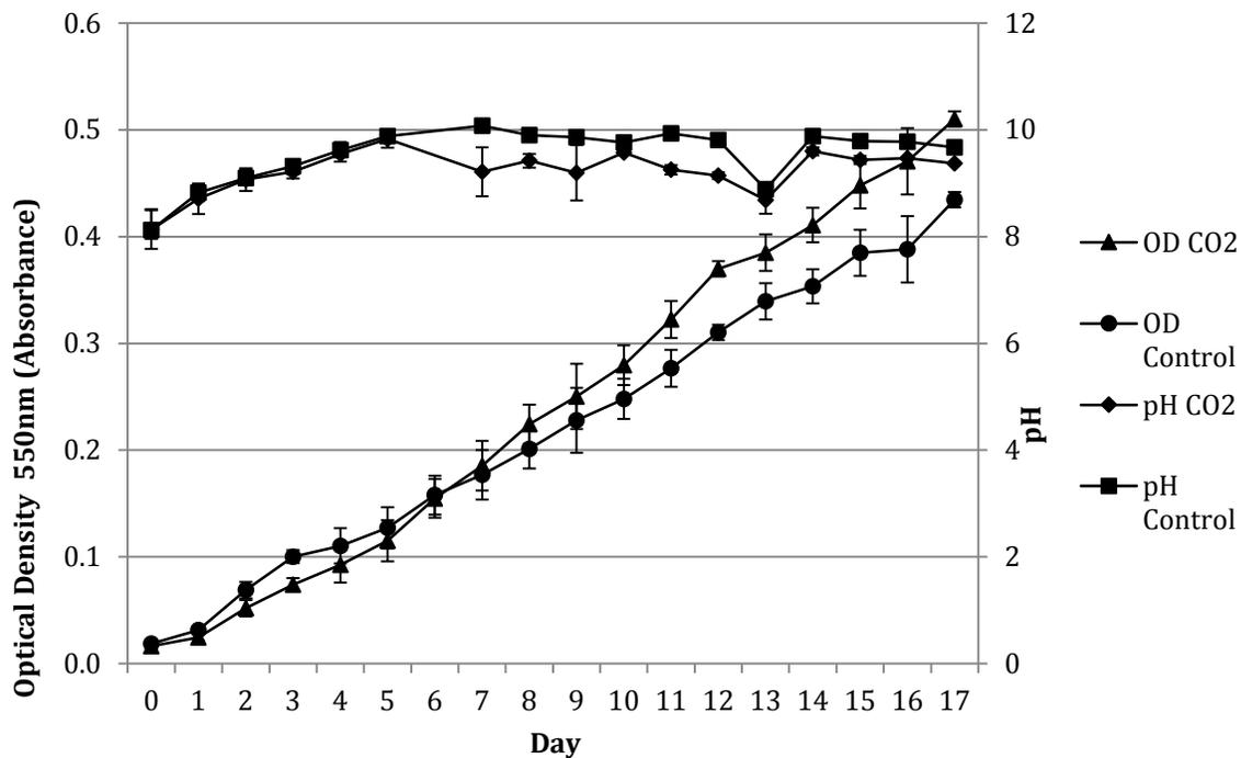
Figure 3. Optical Density 550 nm (Abs) and pH as a function of time in a batch experiment comparing CO<sub>2</sub> supplementation to maintain a maximum pH of 9.5 with control in 10 m<sup>2</sup> raceways.
