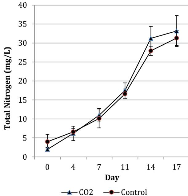
Figure 2. Total Kjeldahl Nitrogen ( $\text{mg L}^{-1}$ ) as a function of time in a batch experiment comparing CO<sub>2</sub> supplementation to maintain a maximum pH of 9.5 with control in 10 m<sup>2</sup> raceways.
