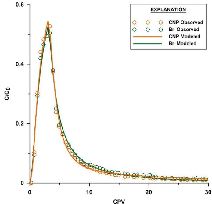
**Figure 2. Breakthrough curves of CNPs and Br for the heterogeneous column with a no-flow matrix. Tailing during the elution suggests diffusion from the core into the matrix and back out.**
