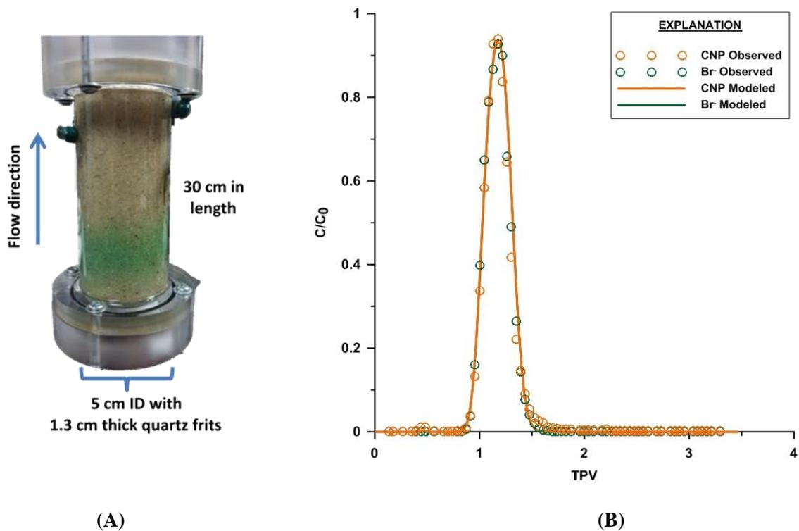
**Figure 1. (A) Illustration of column design. (B) Breakthrough curves of Carbon Nanoparticles and Bromide through the homogeneous column. Note that both tracers are transported nearly identically. The x-axis is time in pore volumes and the y-axis is relative concentration.**
