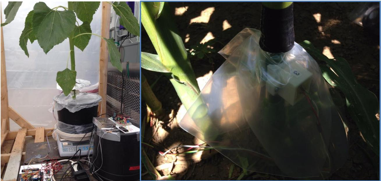
Figure 5. Sap flow gauges being tested on sunflower in the greenhouse (left) and on corn in the field (right). The field deployed gauge is covered with a plastic shield to protect the system from sprinkler irrigation and rain.
