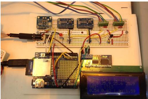
Figure 3. Arduino-based data logging system.
