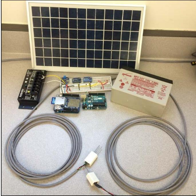
**Figure 2.** A constructed dual-probe heat-pulse sensor for continuous soil moisture measurements. These sensors combine low-cost Arduino microprocessors with heat conducting and sensing probes that are powered by a small solar panel.
