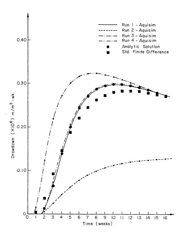
Figure 12. Comparison of drawdowns at 1400m from a pumped well in an infinite, homogeneous aquifer
