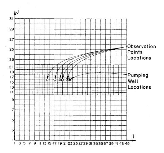
Figure 5. Grid layout used in the standard finite difference solution
