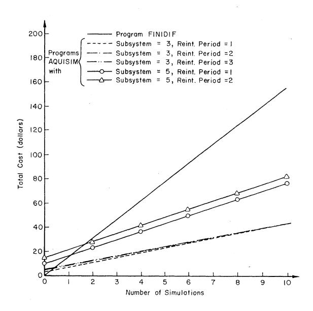
Figure 18. Cost of simulation using FINIDIF and AQUISIM as a function of the number of management strategies
