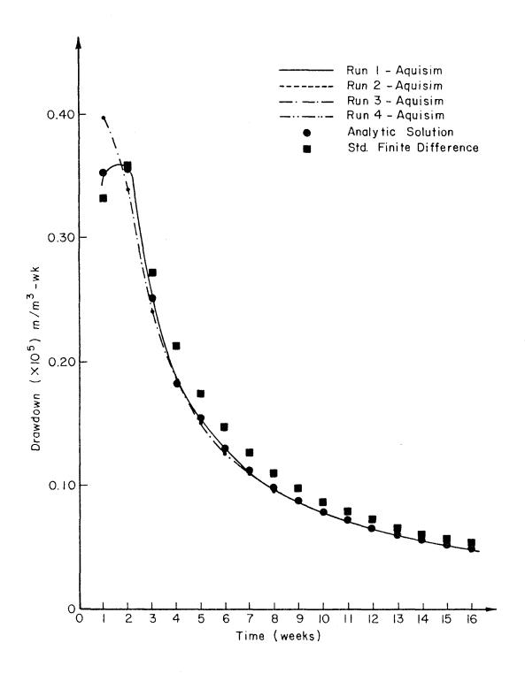
Figure 10. Comparison of drawdowns at  $350\mathrm{m}$  from a pumped well in an infinite, homogeneous aquifer
