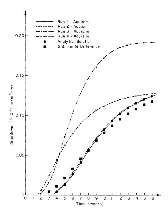
Figure 13. Comparison of drawdowns at 2100m from a pumped well in an infinite, homogeneous aquifer
