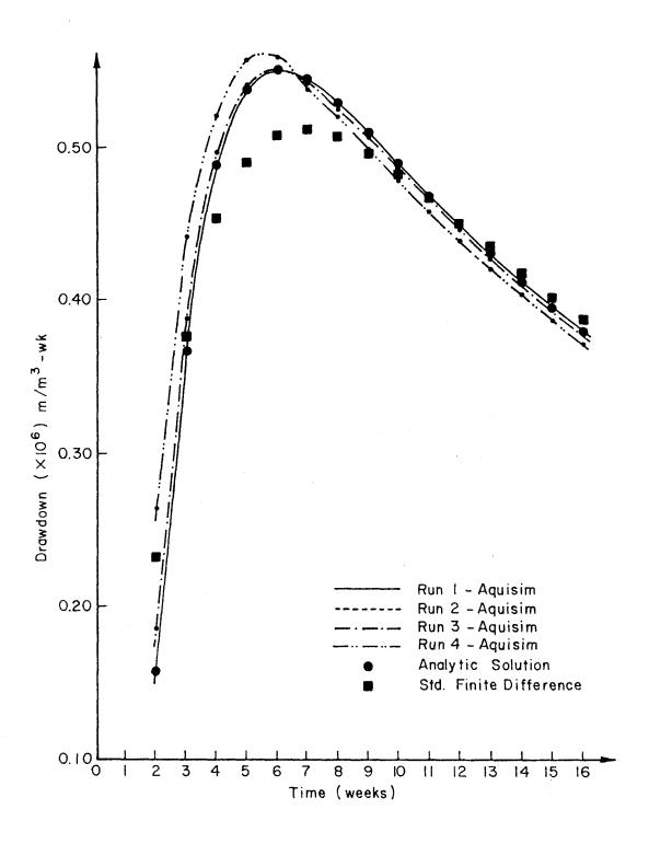
Figure 11. Comparisons of drawdowns at 1050m from a pumped well in an infinite, homogeneous aquifer
