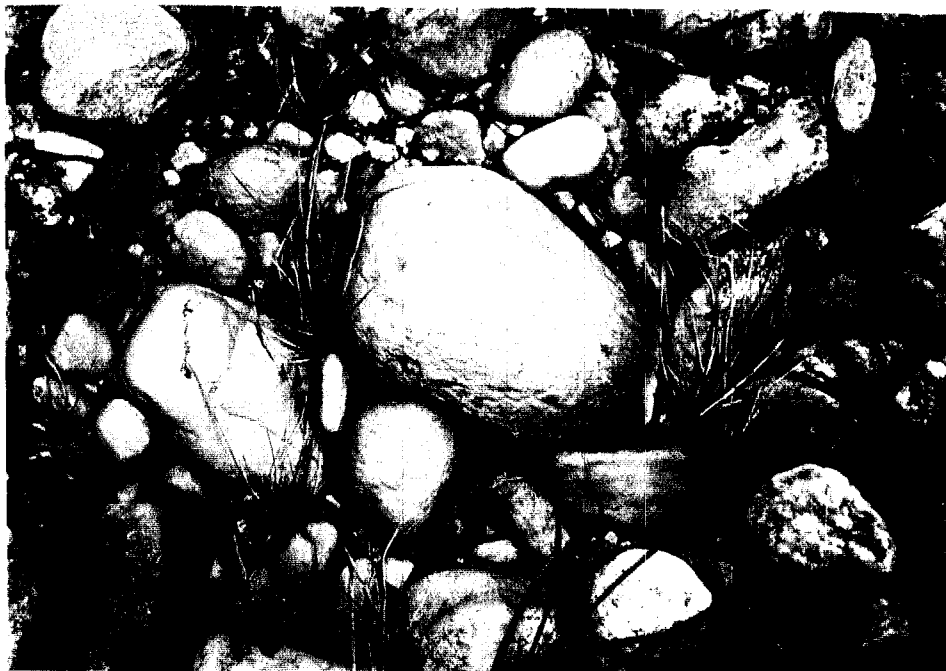
Figure 17 a. Photograph of painted circle (1' in diameter) on exposed channel surface at constrained site after peak flow in 1992. Particles are primarily cobbles with few small gravels.
