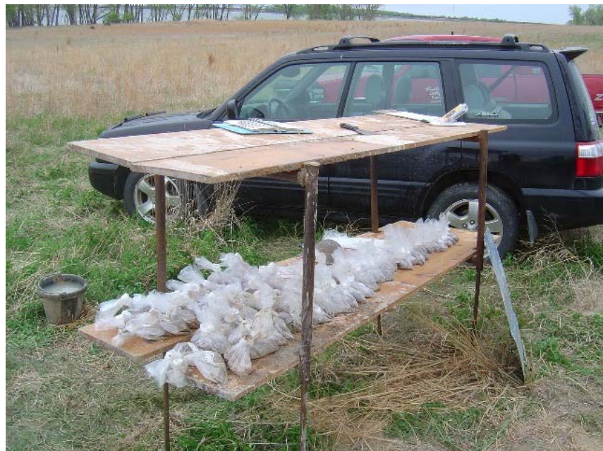
IMAGE 5. Drill cutting samples collected from the deep well at geochemical monitoring well nest 5 in May 2006. Samples were archived at the UNL-CSD.
