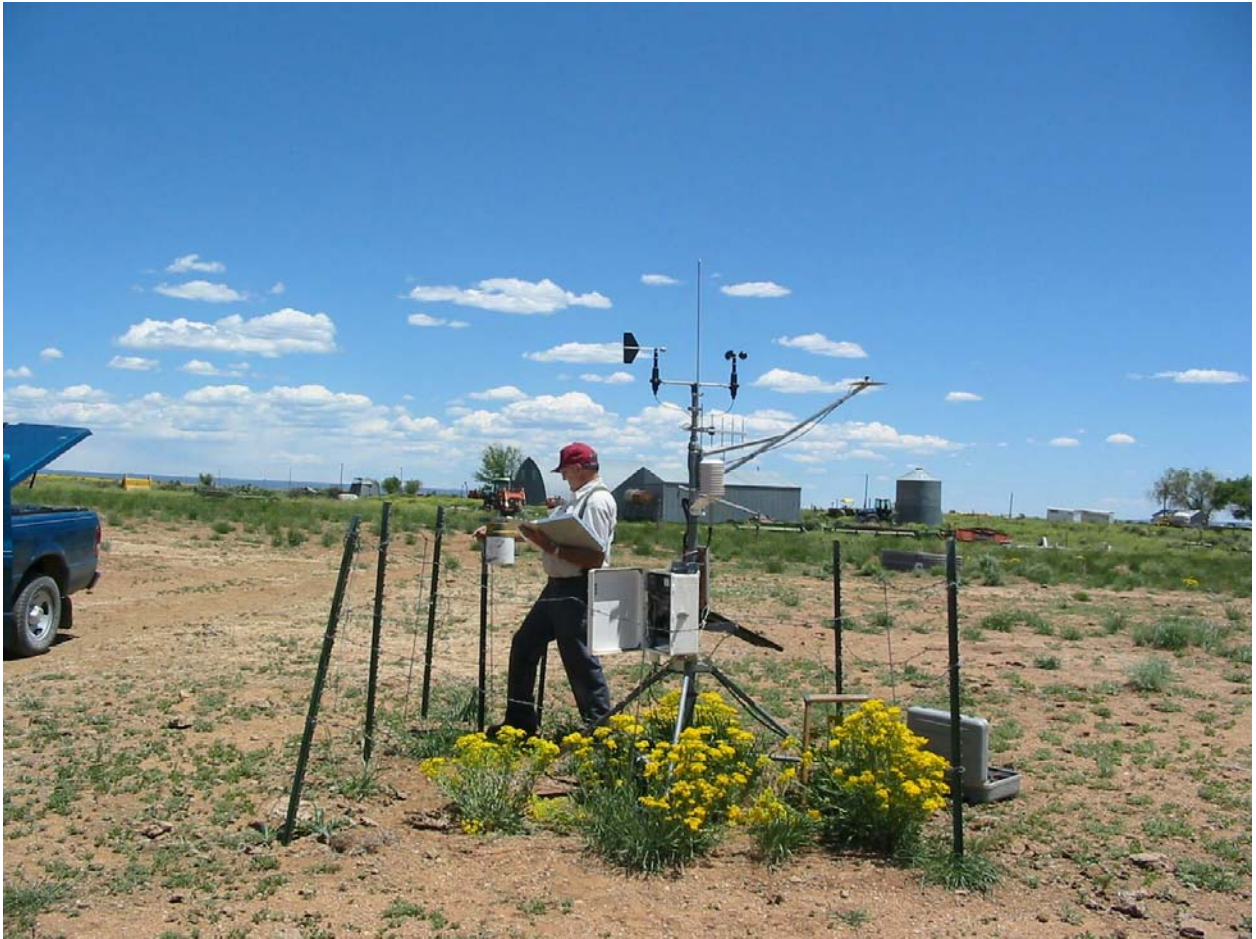
Figure 6: CoAgMet volunteer Dr. Harold Duke (USDA Agricultural Research Service, retired) services the Dove Creek CoAgMet station. Due to sparse ground vegetations, sites like this are not ideal for ET applications.
