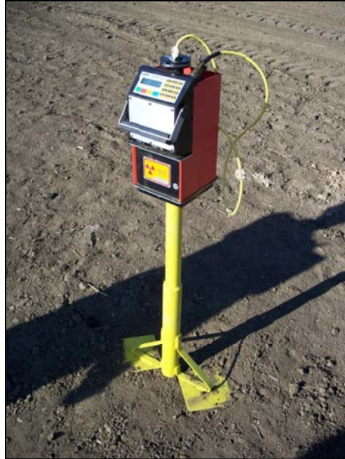
Figure 15. The neutron probe CPN 503DR sitting on top of the depth-control stand
