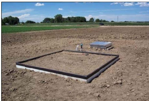
Figure 8. View of the large lysimeter after the soil around it was repacked
