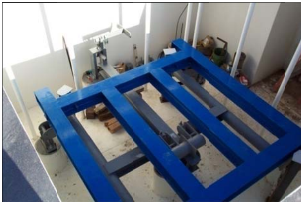
Figure 6. Steel support frame for the soil tank. This photo also shows the scale.
