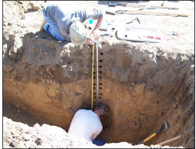
Figure 17. Measuring soil depth before taking soil samples Photo by Kevin Tanabe
