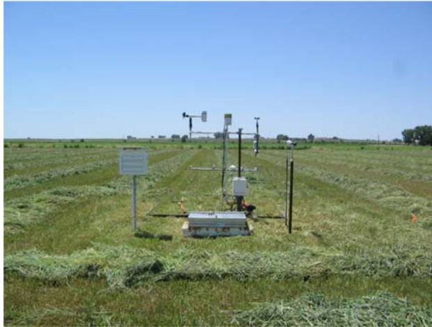
Figure 20. View of the lysimeter and meteorological instrumentation in late June 2007 Photo by Michael Bartolo
