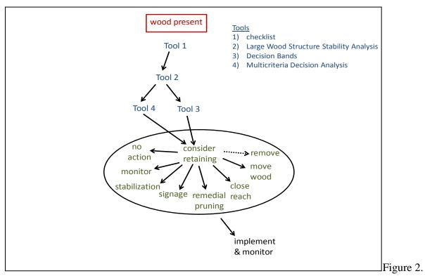
Illustration of the sequence of tasks, and associated tools, which can be used to assess risk created by large wood in streams.
