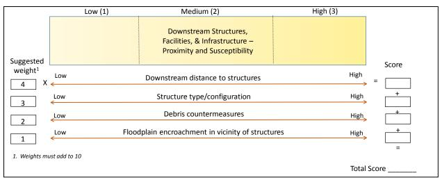
Figure 3G. Decision band for assessing the relative risk to downstream structures, facilities, and infrastructure resulting from the presence of instream wood.
