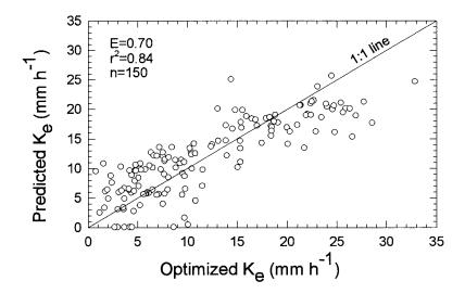
Fig. 1. Comparison of WEPP optimized and predicted effective hydraulic conductivity (K<sub>e</sub>, mm h<sup>-1</sup>) using equations 1 and 2. E is the coefficient of efficiency (Nash and Sutcliff, 1970), r<sup>2</sup> is the coefficient of determination and n is the number of data points.
