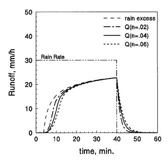
Fig. 6. Effect of roughness on surface storage.
