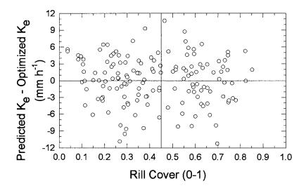
Fig. 2. Difference between WEPP optimized and predicted K<sub>e</sub> using equations 1 and 2.
