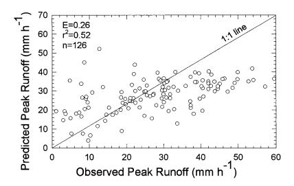
Fig. 4. Comparison of WEPP predicted peak runoff using K<sub>e</sub> values estimated using equations 1 and 2 and observed runoff. The data set of observed peak runoff is from the same plots that equations 1 and 2 were developed from. E is the coefficient of efficiency (Nash and Sutcliff, 1970), r<sup>2</sup> is the coefficient of determination and n is the number of data points. The number of data points shown is 126 because 24 plots had zero predicted runoff.
