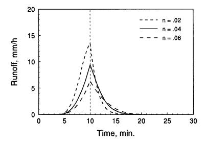
Fig. 7. Effect of roughness for short storm.
