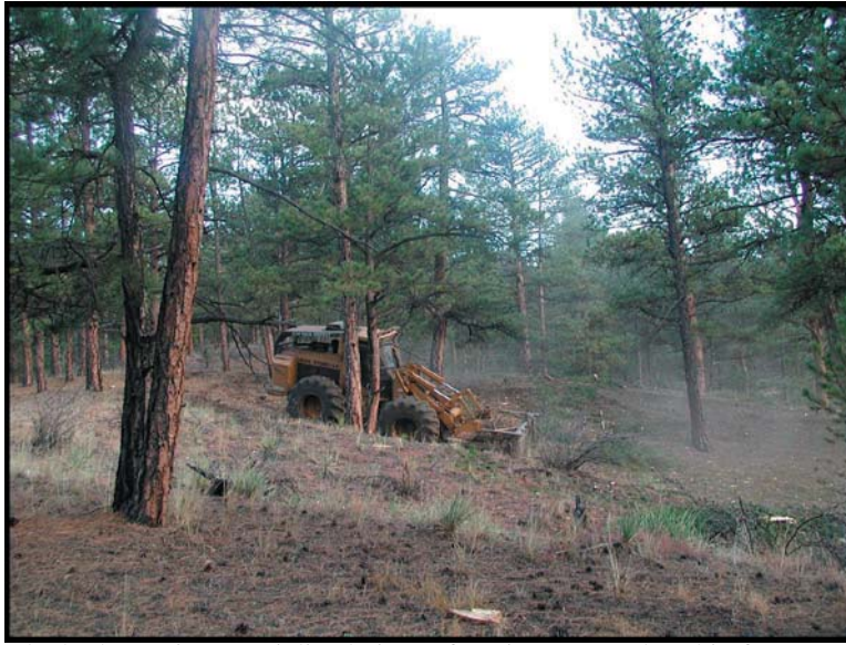
The hydro-ax is a specialized piece of equipment used to thin forests. It also breaks up hydrophobic soils caused by wildfires, which promotes faster recovery of grasses.
