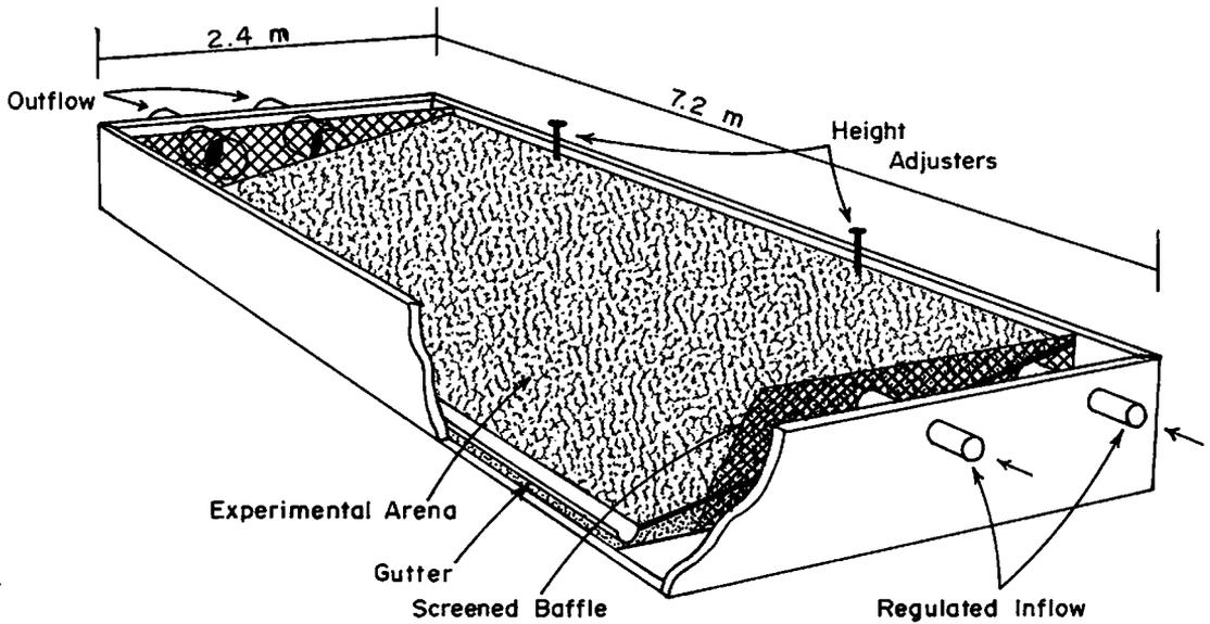
FIGURE 1.—Diagram of the artificial stream channel used for stranding experiments, showing the sloped substrate and refuge gutter on the deep side.
