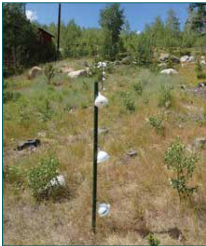
Figure 3: T-posts with double-funnel radiation shields holding the temperature sensors along the hillslope, at the CSU-MC. Photo by Dr. Steven Fassnacht.
