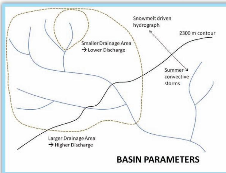
Schematic showing possible basin scale controls on riparian width.
