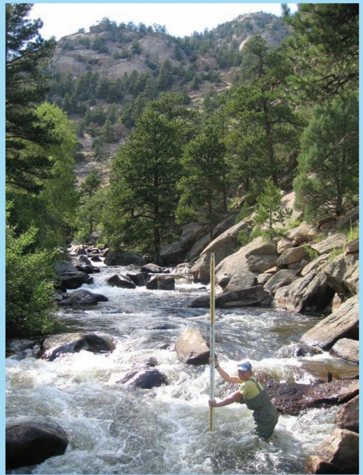
*Lina Polvi surveys a longitudinal profile and valley cross-section in a steep and confined section of the North St. Vrain (west of Lyons, CO).*
