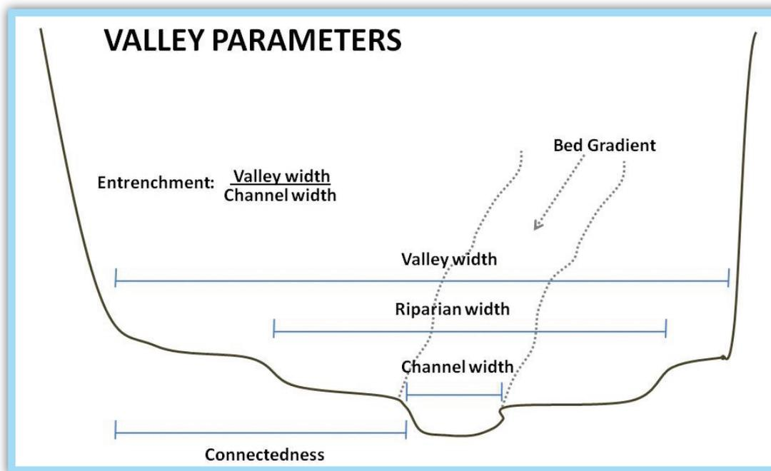
*Schematic showing possible valley scale controls on riparian width.*
