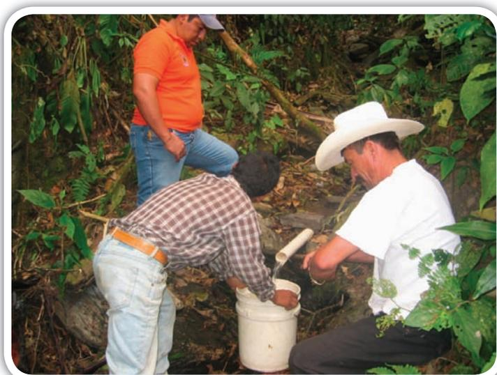
*At the water source for Porvenires, Copán Ruinas, a small dam structure was constructed and flow is being measured by hand.*
