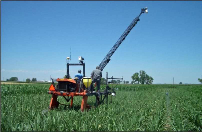
A mobile platform is used to measure crop canopy size, color, and temperature from 24 feet above the ground. (Courtesy of Thomas Trout)
