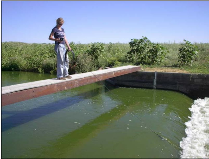
Figure 2.2 Manual Electrical Conductivity Sampling
