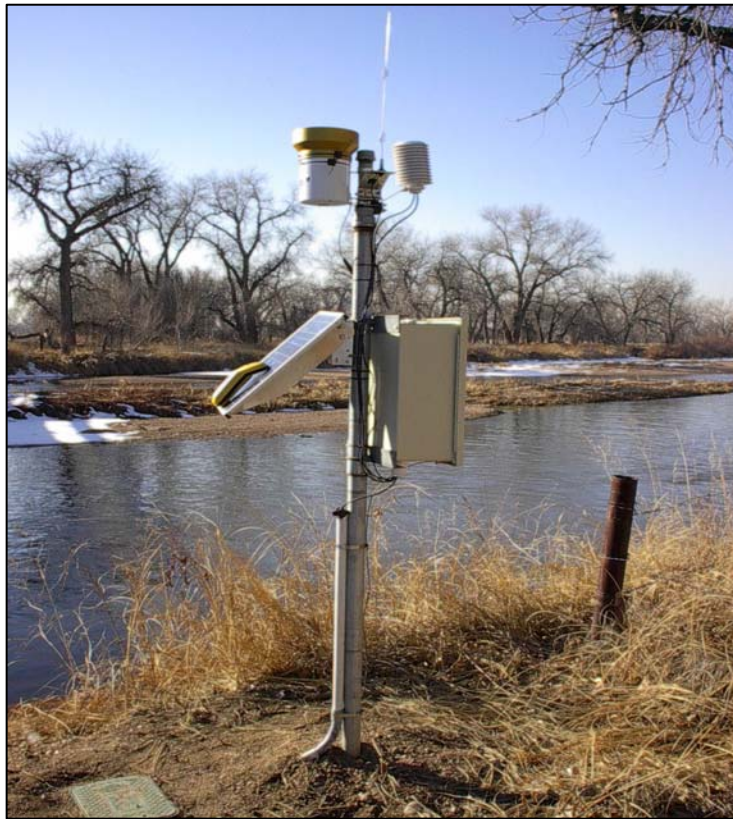
Figure 2.1 Automated Electrical Conductivity Sampling Station
