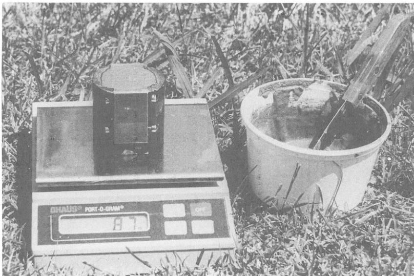
Fig. 14-2. Picture of portable balance used in the field to determine the weight of the saturated soil-paste filling the "Bureau of Soils" cup.
