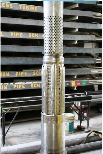
FCV in production (rubber element not installed yet)
