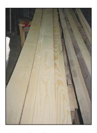
Figure 2. - Clear (no knots), finger-jointed and edge glued ponderosa pine.
