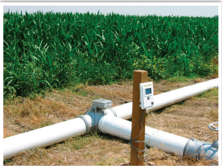
This Hansen displaying logger for WaterMark soil moisture sensors was installed at the top of a corn field near Fowler, Colorado.
