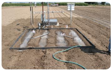
Fig 6: Water being applied to the soil monolith. Photo taken by Michael Bartolo.
