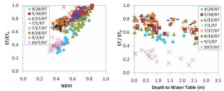
Fig 5: (left) The observed relationship between the evaporative efficiency (ET / ET0) and NDVI at the Swink field site, and (right) the observed relationship between evaporative efficiency and DWT at the Manzanola field site. (Visit the CWRRI website for color version)
