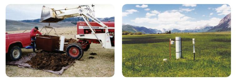
Fig 2: Compensating lysimeters consisted of rectangular steel tanks installed in meadows after excavation of sod and soil. These photos illustrate the installation of the lysimeter (left) and a functioning lysimeter with accompanying weather-monitoring equipment during the growing season (right).
