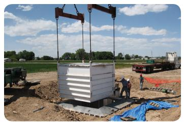
Fig 2: The inner tank plus soil being lowered inside the containment tank. Photo taken by Michael Bartolo.
