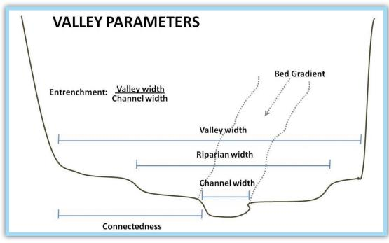
Schematic showing possible valley scale controls on riparian width.
