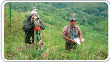
Ben Latham performs a topographic survey in the community of Aldea Nueva, Copán Ruinas, using theodolite equipment for subsequent system design.
