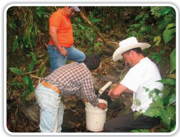
At the water source for Porvenires, Copán Ruinas, a small dam structure was constructed and flow is being measured by hand.
