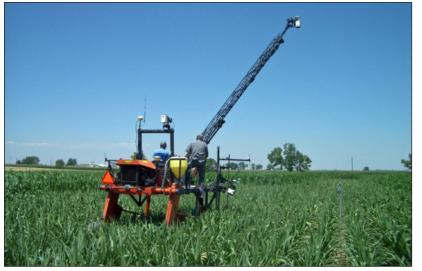
A mobile platform is used to measure crop canopy size, color, and temperature from 24 feet above the ground. (Courtesy of Thomas Trout)
