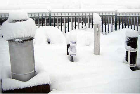
Figure 1. Most precipitation gages do not measure snow very accurately.
