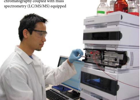
Victor Sam sets up the HPLC (High Performance Liquid Chromatography) for microcystin-LR analysis. GC & LC/MS/MS analysis was done at the Center for Environmental Medicine Analytical Lab at Colorado State University.
