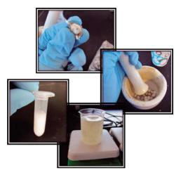
Extraction procedure of active component of the moringa oleferia tree seed. Steps involved deshelling, pulverization, salting and purification. Extraction and experimental procedures performed at the Department of Civil & Environmental Engineering Water Quality Lab at Colorado State University. Courtesy of Victor Sam
