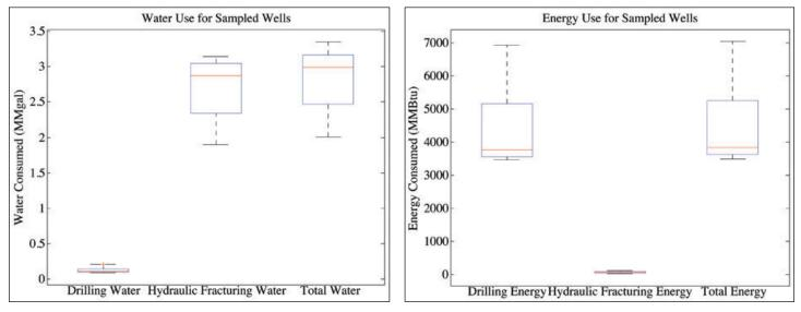
Figure 2. Water and energy use of the sampled wells
