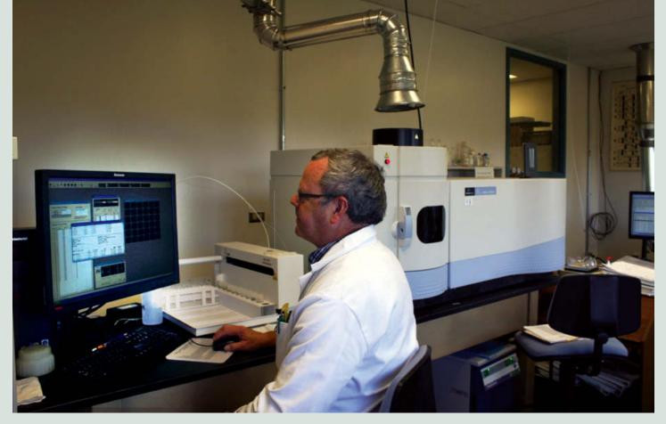
Jim Self operating the inductively coupled plasma-optical emission spectrometer (ICP-OES) in the CSU water lab. The ICP-OES is used for the routine analysis of water samples. Photo by Tegan Deeney
