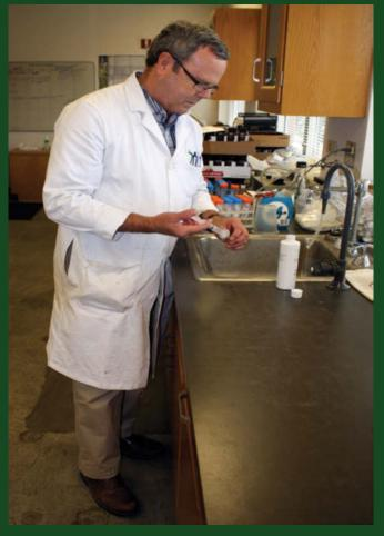
Jim Self filtering a water sample in the CSU water lab to prepare it for analysis. Samples are usually filtered prior to analysis unless the testing requires a non-filtered sample. Photo by Tegan Deeney
