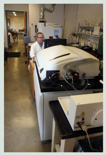
Jim Self operating the inductively coupled plasma-mass spectrometer (ICPMS) in the CSU water lab. The ICPMS is capable of measuring elements at the part per billion or part per trillion level. Photo by Tegan Deeney
