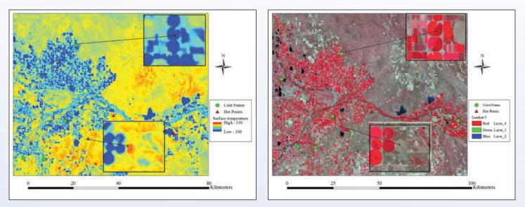
Figure 2. Examples of cold and hot points displayed on surface temperature raster (left) and on the original landsat 5 image (right).
