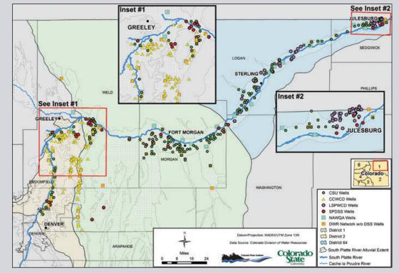
Figure 1. Observation & Monitoring Wells of the South Platte River Alluvial Aquifer
