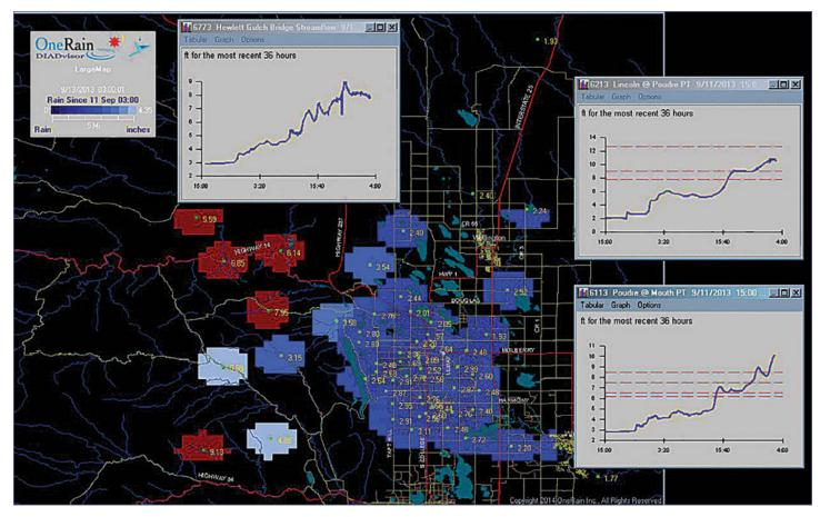
Figure 9. Screen capture at 3 a.m., September 13, 2013 of FWS data-management software showing 2-day rain gauge totals (in inches) and hydrographs (in feet) from three river gauge locations. Pre-established alarm (emergency response) thresholds shown on hydrographs as red dotted lines. Courtesy of City of Fort Collins Utilities
