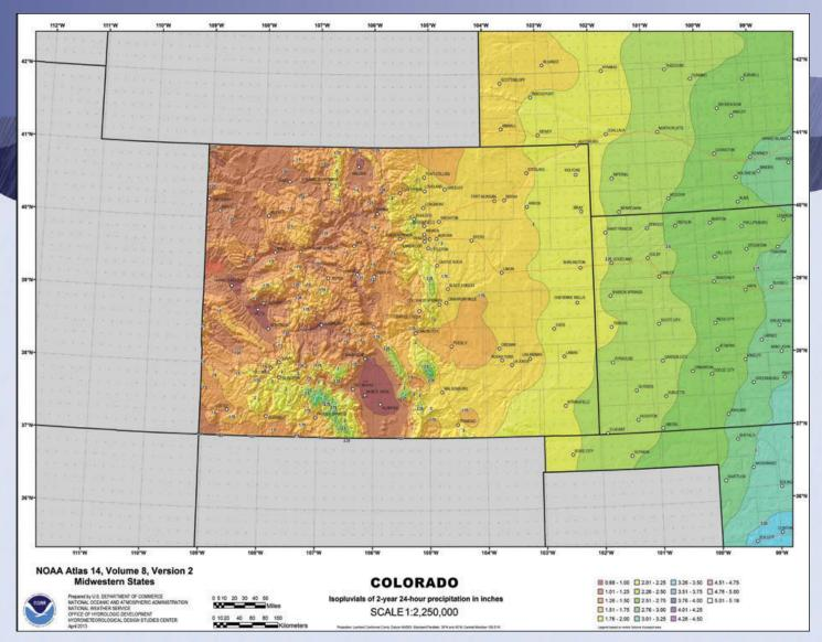
Figure 3. An example of NOAA Atlas 14 data—the Colorado two-year 24-hour precipitation in inches.
