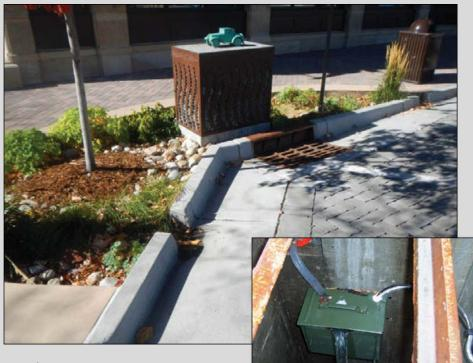
Figure 8. Flow recording equipment and water samples are stored and housed in the decorated cabinet shown.
