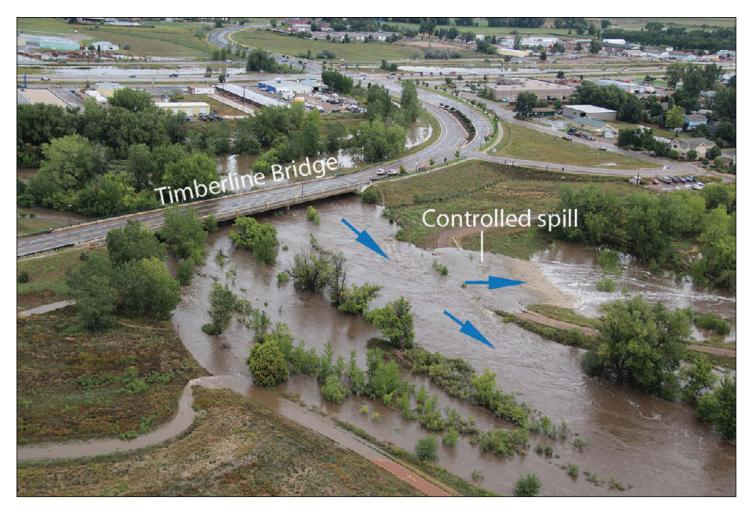
Figure 8. Downstream of the Timberline Bridge on the Poudre River is a controlled spill into Riverbend Ponds Natural Areas. This photo was taken at 12:20 p.m. on Friday, September 13, 2013 during the flooding of the Poudre River and shows the spill functioning as designed. Courtesy of City of Fort Collins Utilities
