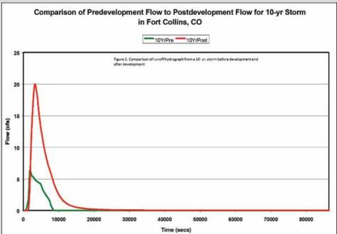
runoff increases by a factor of three. And because the impervious area increases the speed of runoff, the resulting runoff hydrographs from developed area have higher peaks as well as increased volume (see for example, Figure 2). The result is significantly increased channel erosion and destruction of aquatic habitat (Figure 3).
