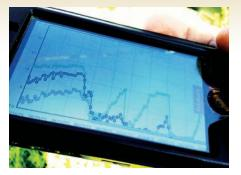
Figure 2. The Sensmit<sup>®</sup> telemetry and software program delivers real-time values of soil moisture so farmers can access their soil conditions from their smart phones.
