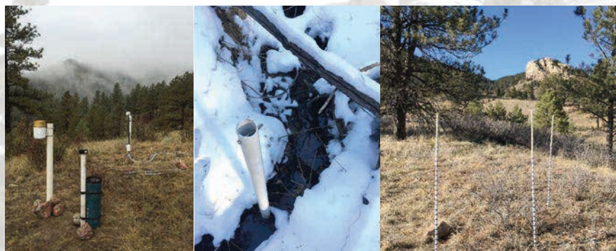
Figure 2. Precipitation and soil moisture instrumentation at Mill Creek (left), water level instrumentation at Lazy D (center), and snow poles for time lapse camera measurements of snow depth at Mill Creek (right).
