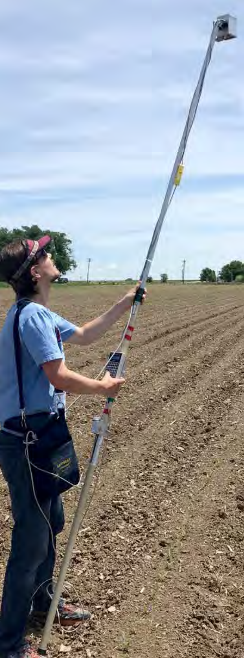
Figure 5. Brian Craig taking readings with the MSR over bare soil. Photo by A.J. Brown.
